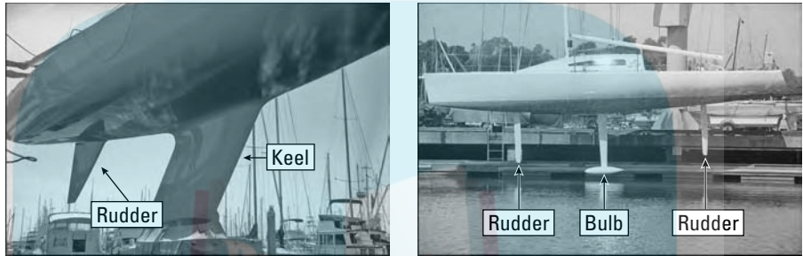
Figure 1-2: Keels and rudders come in different shapes and configurations. The photo at left is common, while the right photo has twin rudders and a canting ballast fin and bulb.
